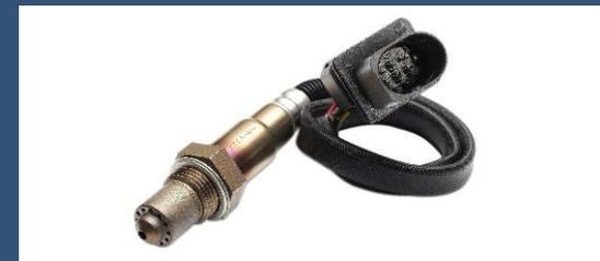
Wideband/Air-Fuel sensors perform the same function as a regular O2 sensor, but they precisely measure the amount oxygen in the exhaust rather than just switching between rich (too much fuel, not enough oxygen) and lean (too much oxygen, not enough fuel). Our Wideband sensors use a more sophisticated sensing element that provides a signal to the vehicle's ECU that is proportional to the amount of oxygen in the exhaust.
